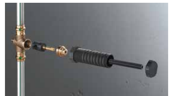
Design of the Easytop concealed free-flow valve
