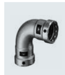
Viega Megapress For steel pipes pursuant to EN 10220, EN 10255, EN 10216-1 and EN 10217-1, in pipe dimensions from 3/8 to 4 inches
