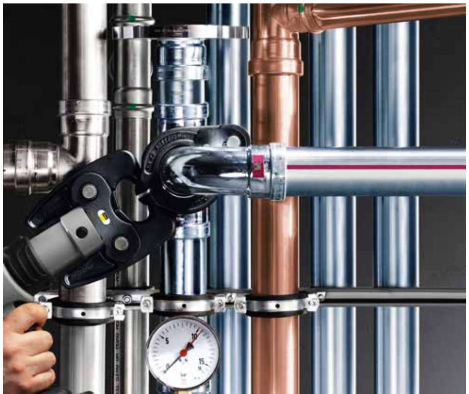
Large dimensions can be easily pressed using the press ring.
