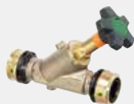
Easytop slanted seat valve (free-flow valve) with SC-Contur - silicon bronze - Raxofix press connection Equipment valve casing and top made of gunmetal or silicon bronze in accordance with DIN EN 1982 and metal evaluation criteria (UBA) (German Federal Environmental Agency), stainless steel valve seat and valve plate unit, spindle transmission, position display open/closed, ergonomic handwheel and closed with medium marking green/red exchangeable, drain plug G¼ with DVGW-test mark Model 5337.5
