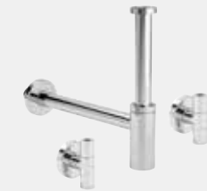
Eleganta set bottle odour trap - equipped with Eleganta corner valve model 5788.45 - chrome-plated brass Equipment 2 Eleganta corner valves, adjusting pipe 200 mm, drain pipe 310 mm, rosette Ø32xØ80xH15 mm Model 5788.4
