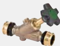
Easytop KRV slanted seat valve (combined free-flow valve with backflow preventer) with SC-Contur - silicon bronze - Raxofix press connection Equipment valve casing and top made of gunmetal or silicon bronze in accordance with DIN EN 1982 and metal evaluation criteria (UBA) (German Federal Environmental Agency), stainless steel valve seat and valve plate unit, spindle transmission, position display open/closed, ergonomic handwheel and closed with medium marking green/red exchangeable, test connection, drain plug G¼ with DVGW-test mark Model 5338.5
