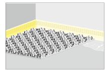
Fig. 41: Lay the Fonterra Base snap plates from left to right. Arrange the film flaps under the snap plate.
