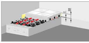
Floor structure Base Flat 12 with Fonterra Base snap plate, smart
