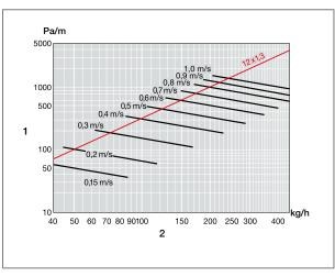
Fig. 32: Pressure loss diagram PB pipe 12 x 1.3 mm
