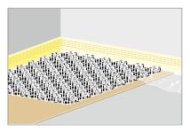
Fig. 43: Laying the Fonterra Base snap plates free of hollow spaces over the entire surface. Arrange the film flaps under the snap plate.
