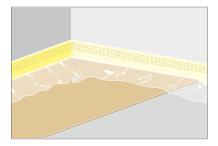
Fig. 42: Lay footfall sound insulation if applicable. Arrange the film flaps on the insulation.
