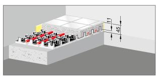
Fig. 28: Floor structure Base Flat 12 with Fonterra Base snap plate, ND 11
