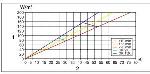
Fig. 36:  $R_{\lambda,B} = 0.15 \text{ m}^2 \text{ K/W}$ Key (1) Heat flow density [W/m2]
