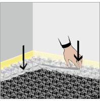
Fig. 74: By means of an edge profile, fix the foil of the edge insulation strip free of tension on the snap plate.
