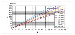
Fig. 58:  $R_{\lambda,B} = 0.15 \,\text{m}^2 \,\text{K/W}$
