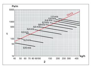
Fig. 54: Pressure loss diagram PB pipe 12x 1.3 mm
