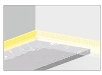
Fig. 72: Lay the footfall sound insulation.
