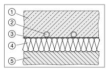
Fig. 69: Systems with pipes within the screed
