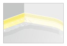
Fig. 71: Lay and fasten the edge insulation strips.
