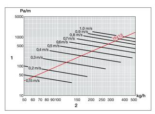
Fig. 59: Pressure loss diagram PB pipe 15 x 1.5 mm
