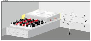
Fig. 51: Installation situation I according to DIN EN 1264-4
