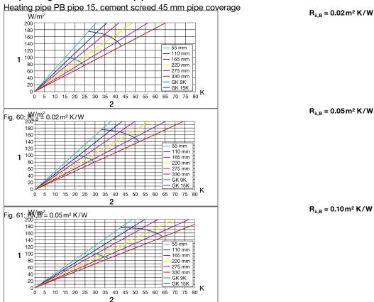
Fig. 62:  $R_{\lambda,B} = 0.10 \,\text{m}^2 \,\text{K/W}$
