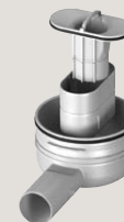
4982.92 Drain for installation heights from 95 mm, drainage capacity: 0.5–0.55l/s, water head seal: 50 mm (can be shortened to reconstruction model)
