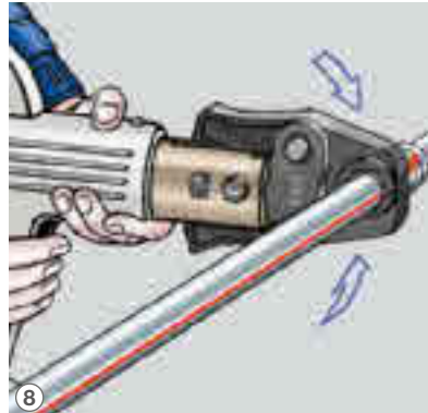
Check the insertion depth and start pressing.
