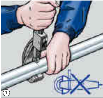
① Cut the pipe to length at a right angle.
