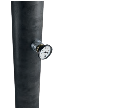
Fig. 39: The steel pipe connection Rp ¾ for thermometers, temperature sensors, manometers, drains or line connections is completed.
