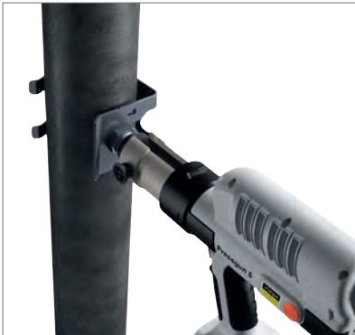
Fig. 38: Now, the press-in branch connector is pressed to the steel pipe by means of the press machine and the positioning aid. This is a fast and clean way of making the connection to the pipeline.
