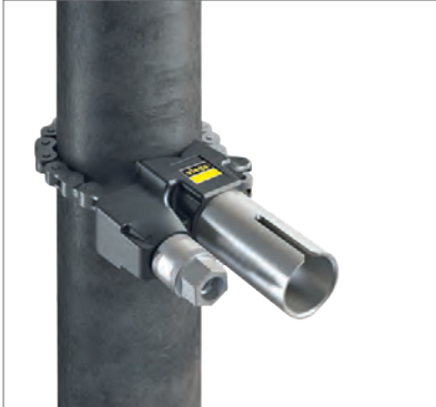
Fig. 36: A special holding device for guiding the drilling shaft is fastened to the steel pipe (1½ to 6 inches) by means of ring or fork spanner.
